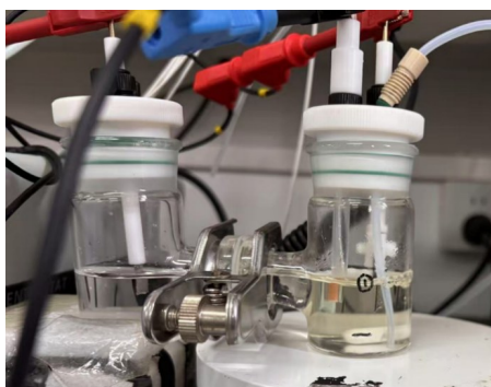
Figure 1 Diagram of the electrocatalytic reduction of NO reaction apparatus
